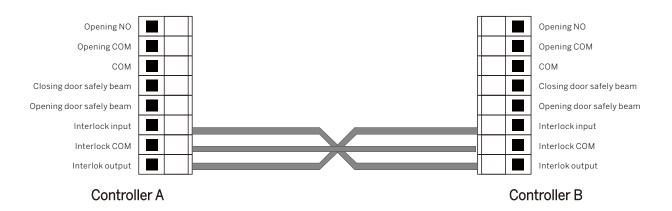
Note: Two doors share same sensor or same signal source, both doors may hold open, in this case, exchange two signal wires of the sensor which is connected with the same controller, it doesn't matter controller A or B.
