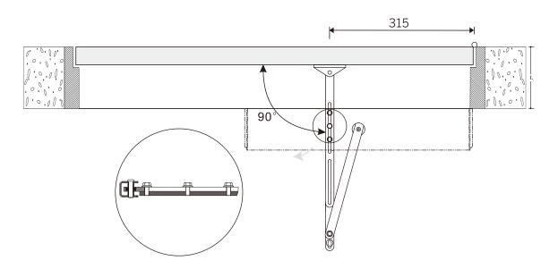
Loosen this three bolts and adjust the push arm length according to the door depth(L) until the angle between the push arm and door panel is  $90^{\circ}$ .
